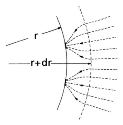
The lines of flux are radial outside r + dr. The concentration of resource is 0 at the surface of the sphere,  $P_{\infty}$  outside the larger sphere of radius r + dr, and some intermediate value in between.
