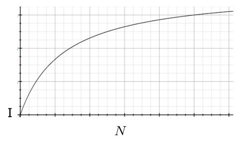
• Given this relationship, we can see that the diffusion current through the patches will reach  $\frac{1}{2}$  its maximum when  $N = \frac{\pi r_c}{r_d}$ . This number can be surprisingly small.
